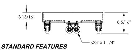
MODEL NUMBER IS DRUM-DP-LD-55-BU OVERALL DIAMETER IS  $\phi$  24 1/4" INNER DIAMETER IS  $\phi$  23 5/8" OVERALL HEIGHT IS 8 5/16" MAX CAPACITY IS 300 LBS MADE FROM HIGH DENSITY POLYETHYLENE HARD RUBBER 3" CASTERS COLOR IS SAFETY BLUE, MUNSELL - 2.5PB 3.5/10 WORKS WITH 55 OR 30 GALLON DRUMS
